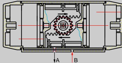
Air to Port B forces the pistons inwards, causing the pinion to turn clockwise while the air is being exhausted from Port A.
