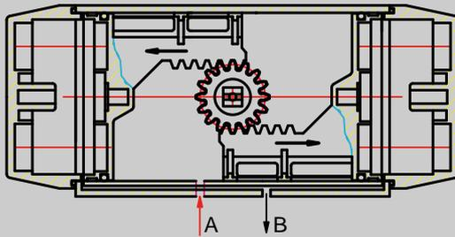
Air to Port A forces the pistons outwards, causing the pinion to turn counterclockwise while the air is being exhausted from Port B.
