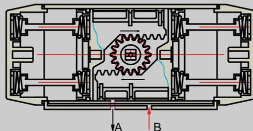
Loss of air pressure, the stored energy in the springs forces the pistons inwards, the pinion turns clockwise while air is being exhausted from Port A.
