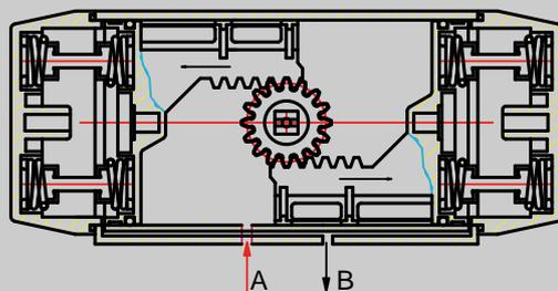
Air to Port A forces the pistons outwards, causing the springs to compress, the pinion turns counterclockwise while air is being exhausted from Port B.
