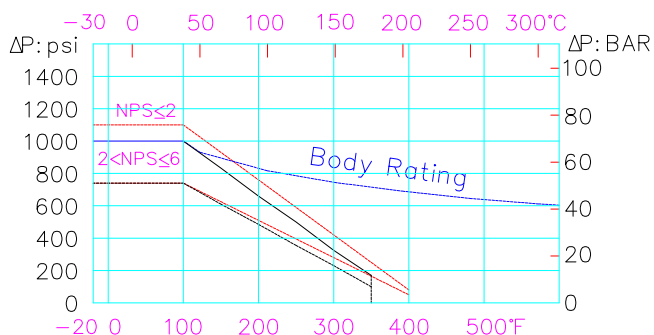
PTFE/R.PTFE Ball SEAT Pressure-Temperature RATING
